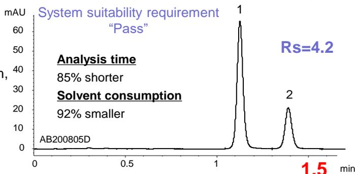
Under UHPLC conditions using a YMC-Triart C8, 1.9  $\mu\text{m}$ , 50 X 2.0 mmI.D. column, analysis time and solvent consumption were reduced by approximately 85–90% while meeting the system suitability requirement and maintaining the resolution requirement of  $\geq 3.0$ .
