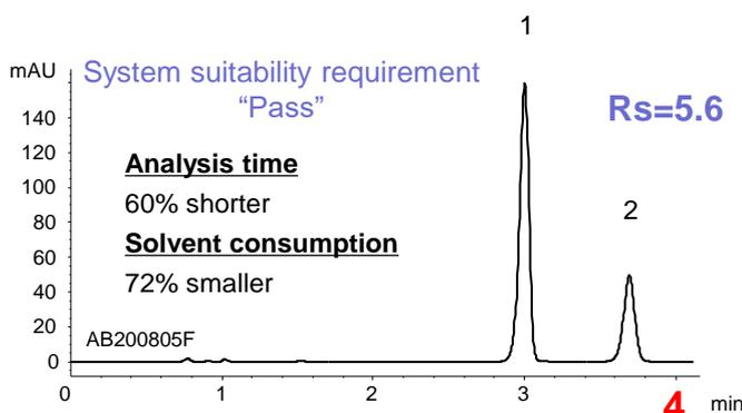
Particle size and column inner diameter were changed to 3  $\mu\text{m}$  and 3.0 mm, respectively. Thus, the column length was set to 100 mm based on L/dp within the permissible range.
